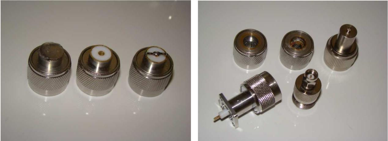
I also made a Short which has no Teflon part included as the electrical length is only the internal "tube" from the reference plane to the shorting plate of 11.5mm with air dielectric only. This should be a fairly accurate Short of a one way delay of **38.33 ps** or **76.66 ps when used in conjunction with setting under CAL kit parameters** . It will be referenced as the ***N 38.33ps Short***
