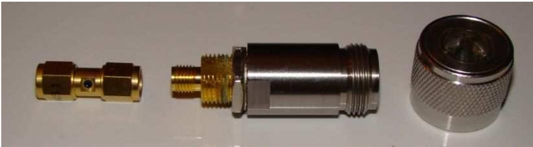
By setting the Port Extension Thru delay to -38.33 ps we can tune the S21 delay so the  $\text{Imag } Z$  is 0 degree and thus position of the ***N 38.33ps Short*** shorting plane by adjusting the Ext. Port1 delay until  $\text{Imag } Z$  is = 0.
