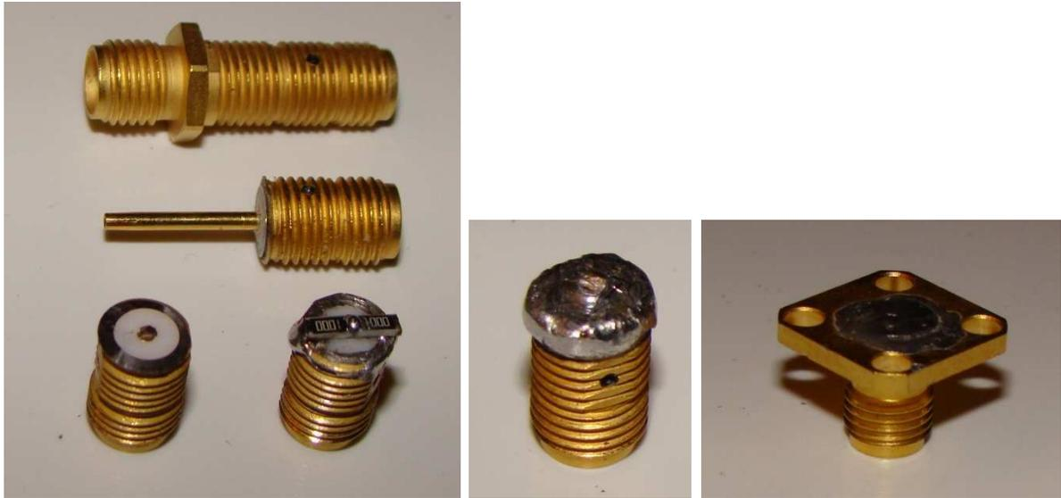
A quite common SMA Panel Jack Flange connector is shown to the right. It has a front to back distance is 9.5 mm and the picture shows it as a Short Adaptor, where a 0.2mm tinned disk is soldered to back and center pin. The distance from front to the internal Reference plane is 2.0mm.
