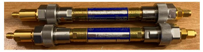
The same calibration coefficients and technique were used on the VNAs (well, the ones that could support it). For instance, the 8720ES does not support inductance correction of the short standard, so the E8364C coefficients definitions were changed to the same ones on the 8720ES. I also used a number of SMA-pin to SMA-socket attenuators (50dB, 10dB, 20dB, 30dB, 40dB) to examine dynamic range.
